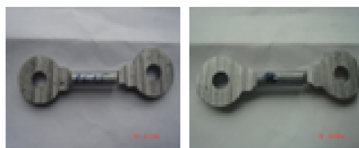
Fig. Specimen tensile testing: (a) atmosphere casting; (b) vacuum casting
