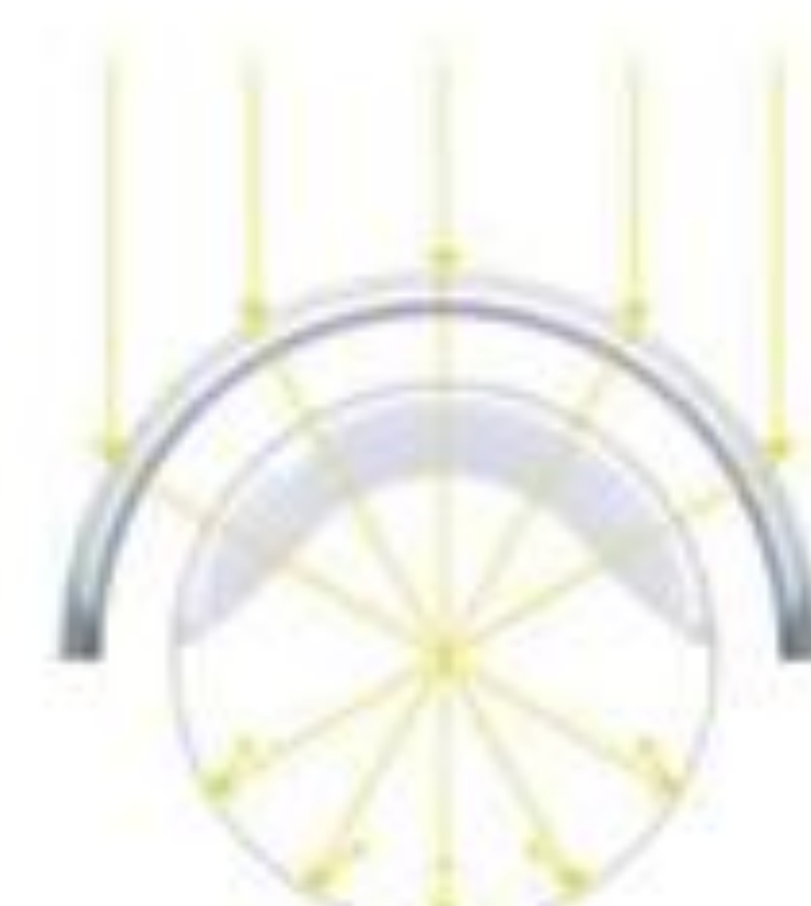
If we put solar panel align in 3-D into the sphere, and guide the light into the sphere through convex, the light will repeatedly reflect till all the energy absorbed by solar panel.
